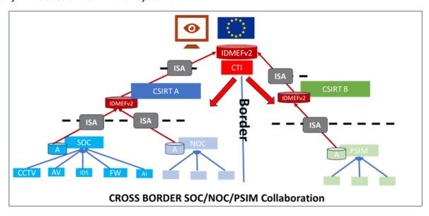
In the diagram above, the ISA modules represent the possible filtering of information shared by SOCs from national SOCs to a European SOC, making it possible to detect combined attacks on several operators at national and European level, as well as the sharing of new "Threat Intelligence".
